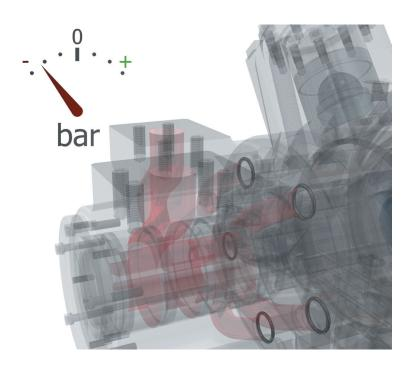
Cavitation can occur due to many different factors. Although it is not possible to make the HMF motor resistant to cavitation, certain features can be added to improve the motor's resistance to short periods of lost port pressure.
